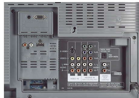
Back side of the Sony Wega HDTV set shows 6 audio/video and two RF inputs. (Courtesy: Crutchfield)
