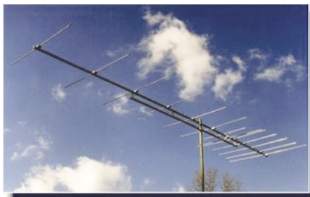
The APS-13 FM Yagi antenna may be the only hope of hearing HD FM stations from 100 miles out. Don't forget to add a good antenna pre-amp! (Courtesy: Stark Electronics)
