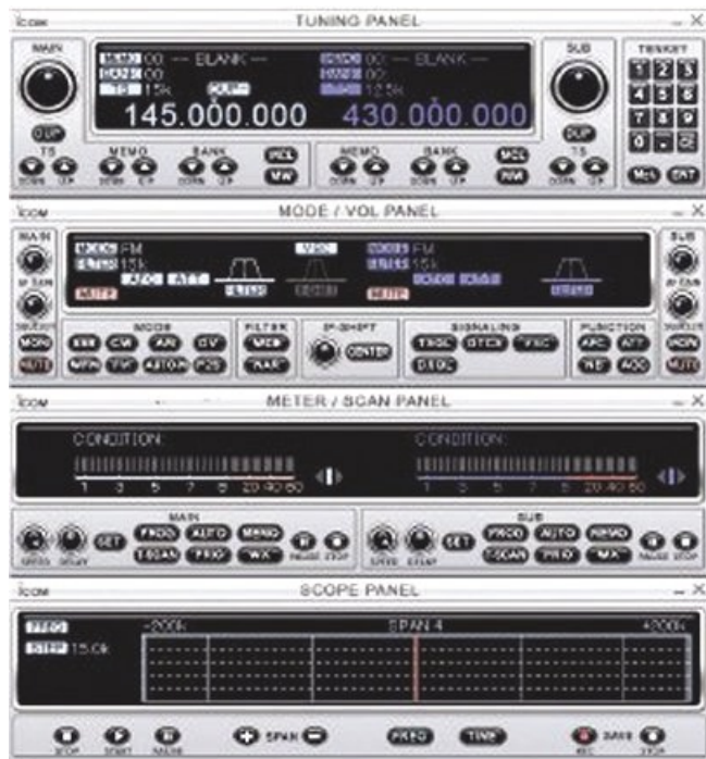
Figure 2 – Seeing Double. The PCR2500 in DualWatch Mode. Notice the two frequencies 145 and 430 MHz being monitored simultaneously.
