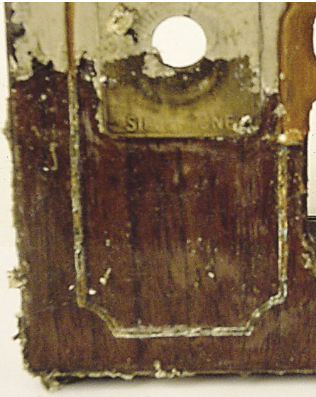
As paint is stripped off, original finish is revealed. Note Silvertone name partly visible on volume control bezel.
