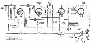
Fig. 1. Circuit of the "International Kadette Universal TRF Receiver." Introduced about 1932, it may have been the first a.c.-d.c. set.
