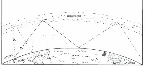
FIG. I. A high vertical angle of radiation results in signals returning to earth relatively near the antenna (a), signals at lower vertical angles return to earth farther from the antenna (b).
