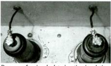
Because of seriously deteriorating insulation, it was necessary to install new grid leads for the r.f. amplifier and mixer tubes -- along with new grommets for the leads to pass through. Tube type markings were added by a previous owner.
