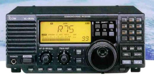
IC-R75 Tune in the world! • 30 kHz - 60.0 MHz • AM, FM, S-AM, USB, LSB, CW, RTTY • 101 Alphanumeric Memory Channels • Twin Passband Tuning (PBT) • Synchronous AM Detection (S-AM) • DSP with Noise Reduction Auto Notch Filter • Triple Conversion • Up to Two Optional Filters • Front Mounted Speaker • Large Display • Well Spaced Keys and Dials • PC Remote Control with Optional Icom RSR75 Software for Windows<sup>®</sup> • And Many Other Features
