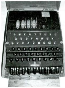
Figure 2 - The pinnacle of ciphering equipment, the German naval four-rotor Enigma machine circa 1944.
