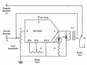
Figure 2 - Schematic for the scanner switch. VSI is wired on its own small PC board, and all other parts are mounted on the cabinet and wired point-to-point.
