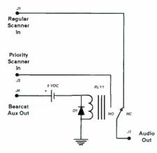
Figure 5 - Schematic for simplified Bearcat version of the scanner switch. This version doesn't need the VC1 because it uses the remote control feature of the BC895xlt.
