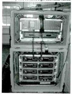
radio power supplies, and interconnect panels. The device also consists of a laptop computer and special software to control the system, interconnect cables, and RF output cables.
