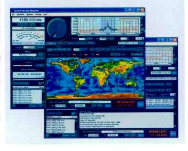
The WR-G33EM receiver offers far more features and facilities than a typical conventional receiver. For example, the real-time spectrum analyzer with continuously variable bandwidth, graphical notch filter and IF recording are just some of the many features which were previously unavailable on a conventional marine radio, in particular at such an affordable price level.
