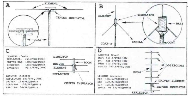
Fig. 1. A half-wavelength dipole antenna (A), a quarter-wavelength ground-plane antenna (B), a 3-element Yagi-Uda beam (C), and a 7-element Yagi-Uda beam (D).
