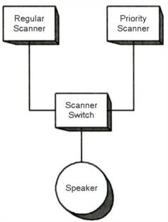
Figure 1 - How to connect the scanner switch. If your scanners feature line-level outputs, you can use the scanner switch with an inexpensive powered speaker. Otherwise use the external speaker connections. You'll have to adjust the volume controls and the VOX sensitivity control accordingly.
