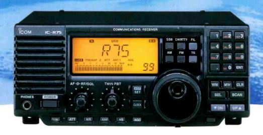
**Tune in the world!** • 30 kHz - 60.0 MHz • AM, FM, S-AM, USB, LSB, CW, RTTY • 101 Alphanumeric Memory Channels • Twin Passband Tuning (PBT) • Synchronous AM Detection (S-AM) • DSP with Noise Reduction Auto Notch Filter • Triple Conversion • Up to Two Optional Filters • Front Mounted Speaker • Large Display • Well Spaced Keys and Dials • PC Remote Control with Optional Icom RSR75 Software for Windows® • And Many Other Features
