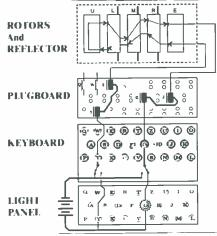
Figure 4 - Simplified circuit diagram of Enigma drawn by Jim Jaeger.
