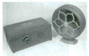
Towards the end of the 1920s, plug-in TRF receivers with simplified front panels replaced the three-dialers. Conetype speakers replaced the horn models.
