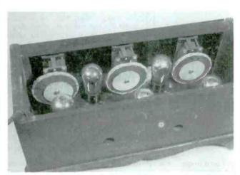
The TRF circuitry required the use of three r.f. coils, each tuned by a separate variable capacitor.
