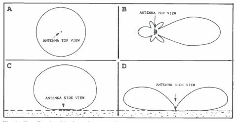
Fig. 1. Non-directional horizontal pattern of a quarter wave, vertical ground plane antenna (A), highly-directive horizontal pattern of a beam antenna (B), vertical pattern of a horizontallymounted antenna showing abundant high-angle radiation (C), vertical pattern of a verticallymounted antenna showing abundant low-angle radiation (D).
