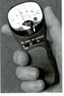
As expected, some environments are packed with radiofrequency (RF) signal sources, and the ZC185 is, after all, a field strength meter; as such, it provides a reading of the aggregate of all signals in the environment. Nonetheless, as discrete signal sources are approached, the readings get stronger.
