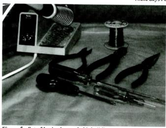
Figure 5 - Set of basic electronic kit building tools
