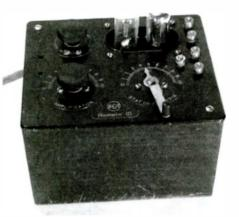
The Radiola III was slightly more sophisticated than the Crosley 50 and boasted a second tube to provide higher earphone volume.
