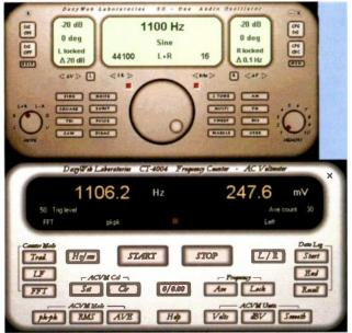
Figure 4 – (Top) The SG One Andio Oscillator is really a very versatile piece of test "equipment". (Bottom) The CT-4004 is an audio frequency counter and an AC voltmeter.
