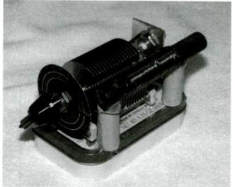
This view of the antenna shows the connections. One end of the pickup loop goes to the center of the connector, the other goes to ground along with one end of the main winding. Ground on the cap is the rotor (frame). The other end of the main winding goes to the stator terminal at the front of the variable.
