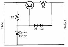
Figure 4 Simple regulator circuit with current limiting
