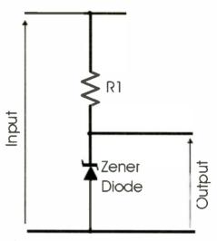
Figure 1 A simple zener diode regulator
