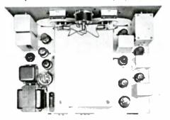
Top view of the HQ-129-X chassis. General layout is almost identical to that of the HQ-120-X.
