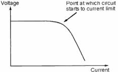
Figure 5 Output characteristic of the regulator with current limited incorporated
