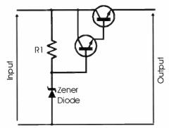
Figure 3 A simple two transistor regulator circuit
