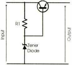
Figure 2 A simple one transistor regulator circuit
