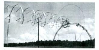
Figure 7-5. Rotatable (in azimuth) 6-turn helical antenna about 45 m long for operation at frequencies around 10 MHz ( $\nu = 30$  m). Note workmen on arch at far end for scale. (Courtes) Electro-Physics Laboratory.)
