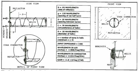
Fig. 1. An axial-mode, helical antenna with equations for determining its dimensions at the frequency at which it is to be operated.
