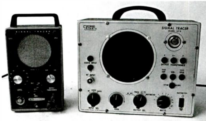
Next month we'll take a look at signal tracers, using the Heathkit IT-12 (left) and the Eico 147-A (right) as examples.
