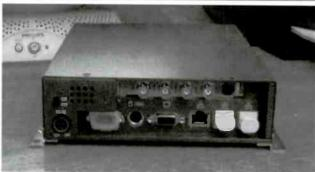
has 248 MB of RAM, a 30GB hard drive and built-in Ethernet, video, USB and serial ports. Windows XP Professional is provided as the operating system.
