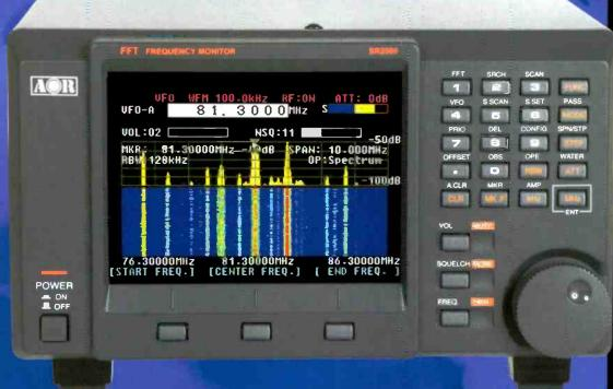
The SR2000 is an ultra-fast spectrum display monitor with a high quality triple-conversion receiver
