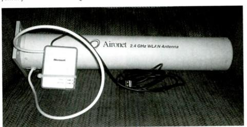
Figure 1: A low cost USB Wi-Fi Adapter modified with 13 dBi Aironet Yagi antenna.
