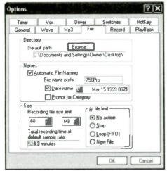
Figure 2: Automatic File Naming is a useful and time-saying feature
