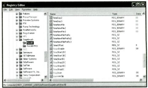
Figure 4: The TimeOffset key and value for RecAll Pro's UTC time-date stamp is added to the Windows Registry with the RegEdit utility
