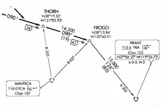
Partial view of a FROGO SIX Departure plate from airport SMF. It shows two VORs with selected radials and two Fixes. (Courtesy NACO/FAA)
