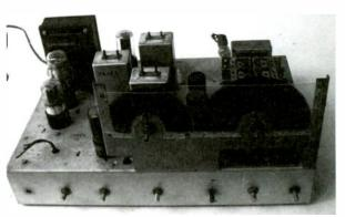
made for automobile finishes Its tubes and dial drives reinstalled, the chassis is ready for had quite a restorative effect on reinstallation in the cabinet. Note replacement plastic window
