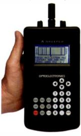
With a frequency range of 30MHz - 3GHz, the X Sweeper can sweep and lock onto a broad range of frequencies in a matter of seconds. The 25 button keypad allows easy access to all functions, provides a direct numerical entry for the center frequency of the sweep range to be easily selected, and easily tunes to a specific frequency in VFO mode. An optional GPS receiver can be added to tag latitude and longitude along with the captured frequency.
