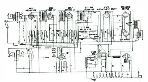
Schematic of the NC-46. Note heater string (at lower right) connected across the a.c. (or d.c.) line.
