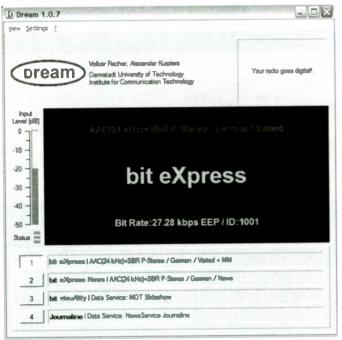
News", and two data streams. The two audio portions are in Parametric Stereo (P-Stereo), and are streamed at a 27.28 kbps raw bit rate. The two data portions consist of slide shows that are transmitted at a 4.08 kbps raw bit rate, called "bit visuAlity" and Fraunhofer's NewsService Journaline®. bit eXpress is listed as transmitting 24-hours a day.
