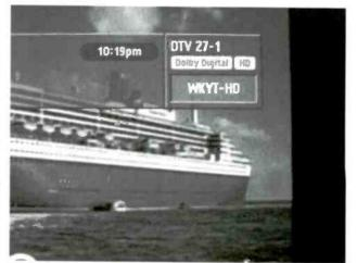
WKYT-DT - PSIP Identification via LG LST-3100A DTV STB
