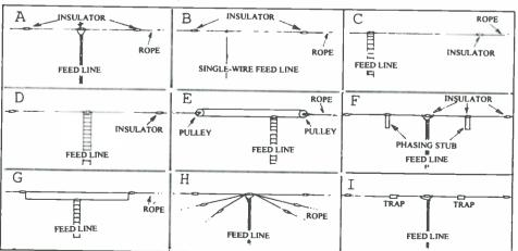
Fig. 1. Hertz, half-wave, center-fed dipole (A), Windom, off-center fed dipole (B), Zepp, end-fed dipole ©), double-Zepp (D), Clothesline folded-dipole antenna (E), Franklin collinear dipoles (F), folded dipole (G), multi-band dipoles (H), trap dipole (I), (antennas not all drawn to same scale).
