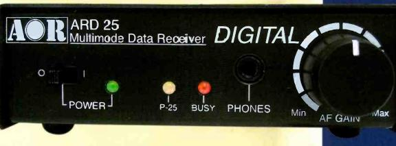
Many high quality receivers were "left behind" when some public agencies began to use APCO Project 25 digital modulation. If your receiver has a 10.7 MHz output port, the ARD25 can translate those digital signals to intelligible audio. In addition, you can also channel your receiver's analog output through the ARD25. It will automatically recognize analog signals and pass them to the ARD25 internal speaker or to an external station speaker. Easy to connect — easy to operate
