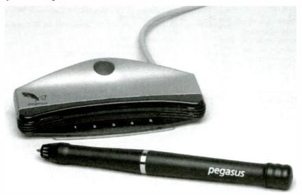
PC NoteTaker consists of the base unit/clip, a digital pen, and PC NoteTaker Software.
