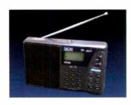
The display indicates station name, used frequency, field strength and the number of service components of the received DRM signal. Additional information transmitted will be displayed if available. The station can be selected by directly entering the frequency using the numeric keypad.
