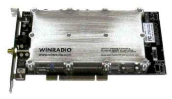
The G303i PCI-card receiver is designed with maximum reliability and performance in mind. Not a single tunable part has been used in its design. There are two high-performace DDS units, and thousands of ultra-miniature surface-mount components delivering a truly stunning performance.
