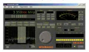
The G303i control panel features no less than seven different methods to tune the receiver. There are additional features such as a real-time spectrum analyzer, three scanning options, a highly accurate S-meter displaying signal strength in absolutely calibrated user-selectable units, sweeping wide-band spectrum scope, powerful memory facilities, and many others.
