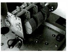
Tuning capacitor assembly "floats" on rubber grommets. Rod at rear of capacitor (lower left) slides through grommet on angle bracket. At right is a portion of the front capacitor mounting bracket showing one of the grommets on which it rests.
