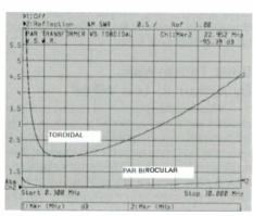
This graph compares noise reduction using the PAR binocular core transformer compared to the customary toroidal core.
