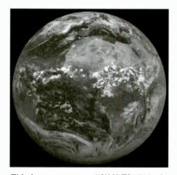
This image, courtesy EUMETSAT, is the first of the new LRIT (Low Rate Information Transmission) format being transmitted currently by MSG-1 (Meteosat Second Generation) as part of the test program before the operational phase starts next year. It shows channel 13 (this is channel 1 visible-light) image from 1145UTC on July 7. LRIT will replace WEFAX on all WXSATs in due course. (see page 90)
