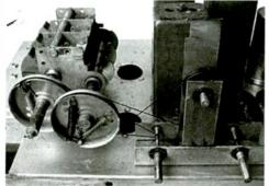
Main tuning and bandspread drive system prior to restoration (left) and after chassis painting, capacitor cleaning and drive restringing. Note extra spring added to bandspread dial drum (see
