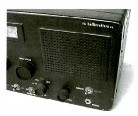
Speaker grille of the S-40B is not a separate piece as in the earlier versions, but is formed from the metal of the panel itself. The "h" logo has been eliminated.
