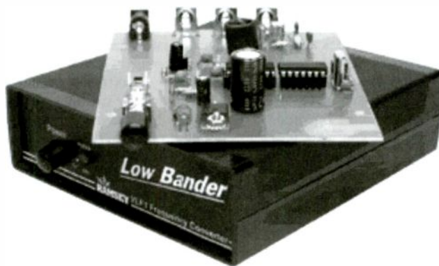
The Ramsey VLF1 is a receiving converter for the frequencies below 400 kHz.
