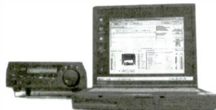
DRM software receiver with commercial HF receiver as front-end
