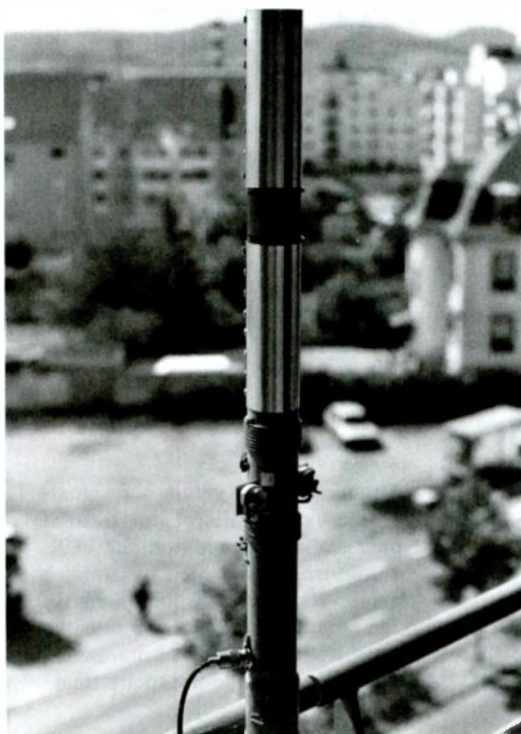
Fig. 3 – Photo of typical EH antenna constructed by Martial Roux, F5IXU (used with permission).
