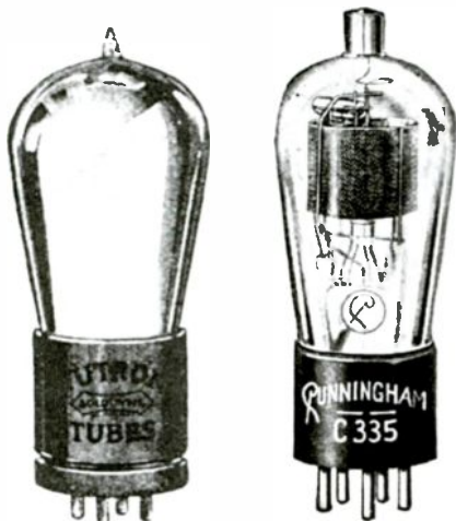
At left, early-20s tube with tip seal, brass bayonet-lock base and stubby pins. At right, late 20s tube with grid cap, Bakelite base and long pins.
