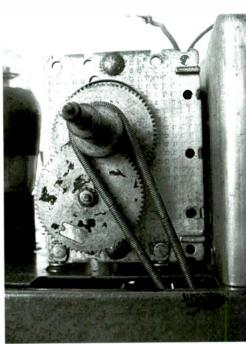
Front of tuning capacitor showing drive gears and top portion of drive spring.
