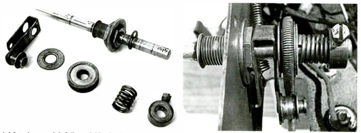
At left, tuning control shaft dismantled for cleaning and evaluation (see text). Replacement for missing "D" clip can be seen temporarily sitting in its groove on right-hand portion of shaft. Reassembled shaft is shown at right as installed in set. Bottom of drive spring is seen at center, idler tension spring is at left, just behind front panel.
