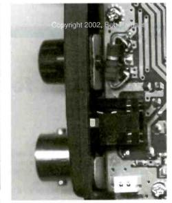
threshold by adding a small, 2200 ohm resistor across the outer two contacts of the squelch potentiometer. Jim used a 3300 resistor instead.
