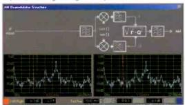
The Professional Demodulator (optional) includes interactive block diagrams for all modes, with two real-time spectrum scopes and THD and SINAD measuring facilities.
