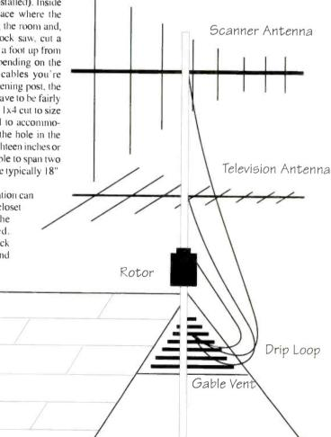
Don't Forget the Drip Loop! Before wire or cable comes into the house from above, such as antennas on a tower, let the cable go below the entry point to allow rain to drip off the wire and not run into your attic.
