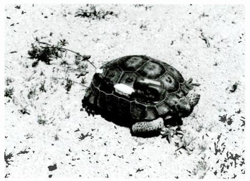
At a peak power level of about 1 milliwatt, pulsed 70 times a minute, the tag on this tortoise will stay on the air for up to two years. The entire package weighs 35 grams and is encapsulated with a desert-proof coating.
