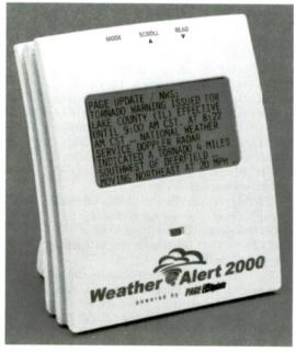
an eight-line backlit LCD screen for displaying text messages and a zoom capability to double the text size, low-battery indicator, message-full indicator, and mute mode.
