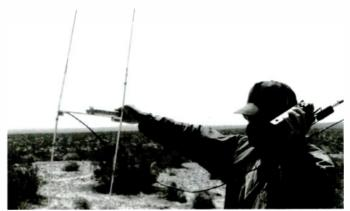
such as hawks. At night, A researcher uses a Sony multimode receiver and attenuator to track they take flight to feed pulsed signals from tags on desert tortoises in California.
