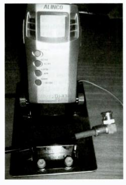
count all the times my handheld radios have fallen over. This is the solution. Some stands even come with a BNC pigtail and a counterpoise ground wire. These are also useful for desktop multimeters
