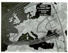
Footprint of Ku band beam showing the extent of the coverage, from northwest England to well into eastern Europe (Loral)
