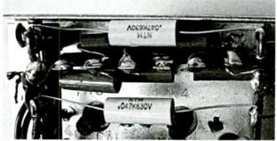
Five resistors wired in series on terminal strip (between the two light-colored capacitors) substitute for burned-out R28 (see text).
