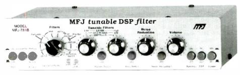
An array of outboard electronic products can improve AM band reception (Courtesy: MFJ Enterprises)
