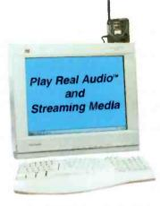
The FM Transmitter is simple to use. Just plug the transmitter into the headphone jack or line out of any audio device and set the frequency of choice (88-108 MHz). You can listen to streaming audio from your computer over your home ste-
