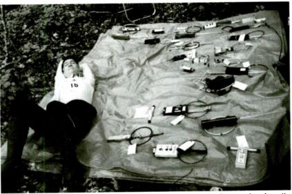
Bob Frey WA6EZV of Ohio catches a quick 40 winks before his late starting time. On the impound tarp are a wide variety of home-built and commercial 80m RDF sets, including air loop and rod antennas.
