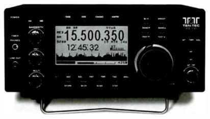
While the bar graph S-meter is calibrated for the conventional 50 microvolt signal equaling S-9, the entire meter is compressed into a one-inch space, with each 1/8-inch reticle division representing nearly 4 S-units (20-24 dB) of signal level change. While an adjacent numeric readout in 1/8-inch characters is provided, it is distracting to have to refer constantly to a changing number to get a fix on relative signal strengths. But it does provide reference levels.
