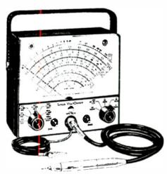
Senior Voltohmist measures up to 1500 d.c. volts in seven ranges; 1500 a.c. volts in seven ranges; 1000 megohms in seven ranges.
