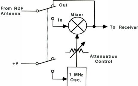
An offset attenuator is similar to the front end of a superheterodyne receiver, where the incoming signal is shifted to an intermediate frequency. In this case, the output signals are at the input frequency plus and minus the oscillator frequency, at levels controlled by the attenuation potentiometer.
