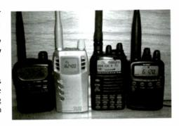
Icom R series have very broad band capabilities. Most impressive is the cost. The R-2, and Yaesu VR 120 are well under two hundred dollars. The Yaesu VR-500, and Alinco DJ-3X are around \$225. These radios hear from 500 kHz to above 1 gigahertz. True, they do not follow trunked 800 systems, but what do you expect for under \$200? They are even computer programmable. Hove them so much. I own all four! See Photo.
