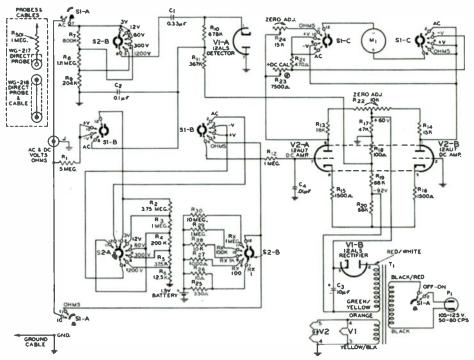
Schematic diagram of the Junior Voltohmist. Note: 12AU7 dual triode is used as a two-stage d.c. amplifier.
