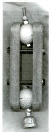
Figure 6. Partially assembled bracket showing golf balls sandwiched between wooden arms
