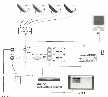
Making connections on the ST7700. Now featuring polarity controls and dish drive connections, DiSEqC switch control, S-VHS out, and channel 3/4 modulator this receiver also converts MPEGII PAL format (courtesy smallear.com)
