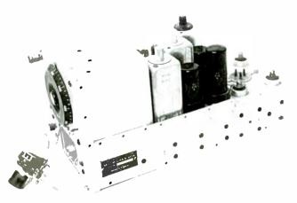
BC-453 with top enclosure removed. Front adapter plate has also been removed for inspection of wiring.
