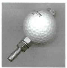
Fig 2: Golf ball with bolt, lock washer, and two nuts.
