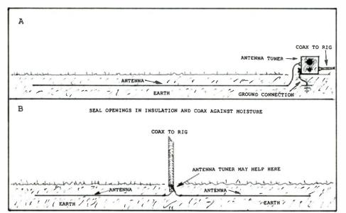
Fig. 1. An underground, or on-ground long wire antenna (A), and an underground, or onground halfwave-dipole antenna (B).
