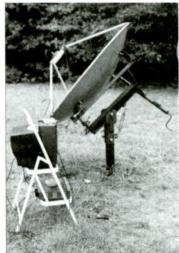
4.5' surplus spun aluminum dish with analog receiver using a C-band LNBF (courtesy author)
