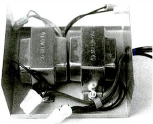
Interior of isolation transformer cabinet. Tied-together 12-volt secondaries are at upper left; their unused center taps are at upper right. Line Transformer voltage input and output connections are below.
