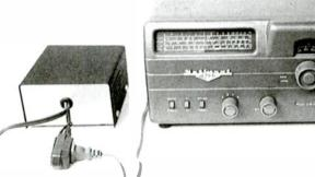
The completed isolation transformer as set up to power the completed SW-54 for a final "smoke test" of both units.
