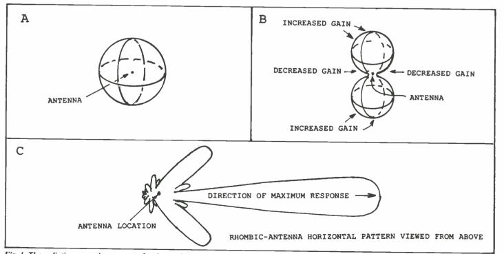
Fig. 1. The radiation-reception pattern of an isotropic antenna: (A) Squeezing the isotropic antenna pattern to give it some directionality, (B) One of many radiation-reception patterns which can be produced by appropriate antenna design.
