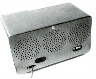
Refinished back from junker set fits nicely and matches well. Line cord runs through opening formerly occupied by interlock plug (see text). Earphone pin jacks are just to the right of the opening. Antenna and ground connections are at far right.
