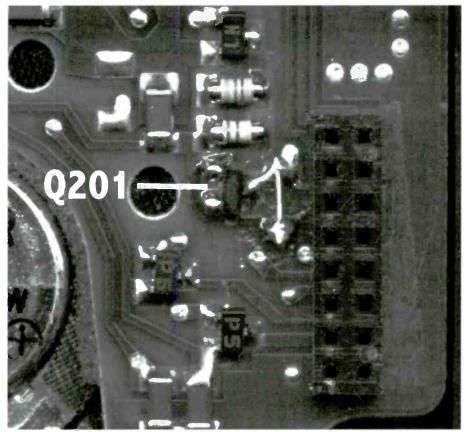
Figure 3. Transistor Q201 location on BC200XLT Micom board.
