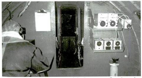
A typical SCR274-N installation (at right) in a B17 radio compartment. Transmitters and antenna coupling unit above; receivers below. Photo courtesy Bill Fizette.
