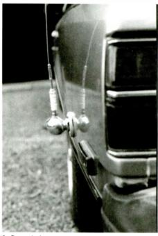
2) Same ball mount with a 5/8-wave, two meter whip. Replace with a 102" steel whip for enhanced SW coverage.
