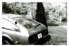
1. Ball mount antenna provides base for a variety of useful mobile antennas. Here a ten meter whip is mounted which also provides good coverage of the higher frequency SW bands.
