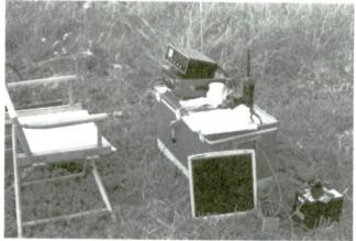
Field Day 2001 gave me an opportunity to try out some minimal station ideas. The entire station including transceiver, transmatch, battery, solar panel, associated cables, wire and microphone fit nicely into the cooler with room for lunch. (Courtesy Author)
