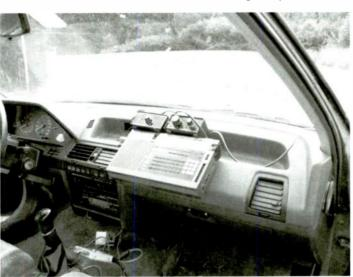
receiver on a large outdoor long wire An "after" photo of the SWL equipment installed in the car
