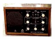
The Grove SP-200C offers variable-bandpass notch/peak function, separate bass and treble equalization, adjustable-threshold pulsenoise clipping, selectable-hold-time recorder activation, audio level, variable-hang noise squelch, and amplification. Processed sound is available through the high quality internal speaker, or from a headphone jack for secure installations or concentrated monitoring in noisy environments.
