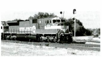
Now owned by CSX, this former Conrail model SD8MAC locomotive generates 5000 HP and is equipped with DP, allowing it to be remotely controlled.
