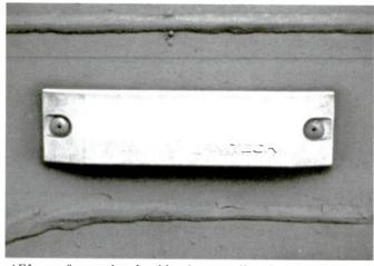
AEI tags, fastened to the side of every railcar in the nation, have automated the process of tracking cars and shipments.
