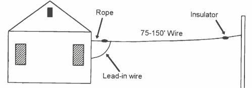
Figure 1. Random wires offer good all-around performance for receiving, and should be a part of any listener's antenna farm.
