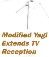
The new TERK TV35 is a combined VHF/UHF outdoor antenna that is designed to extend reception into the fringe areas of TV reception (with an amplifier). Ten antenna elements are designed to deliver high gain (VHF 0-4dB and UHF 2.5-8.5dB) at its operational bandwidth of 54 to 806 MHz. It measures 76-7/8 inches wide by 38-1/2 inches long and weighs a mere 2.65 lbs.
