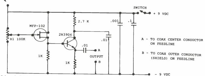
Fig. 1. Schematic diagram for the active antenna discussed in the text.
