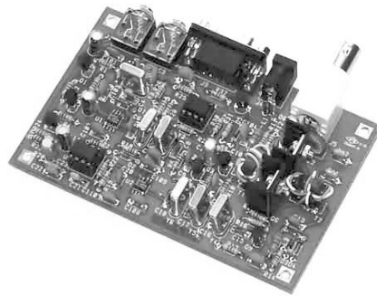
The Warbler is a simple kit that gets you started on 80 - meter PSK31 – NJQRP Club
