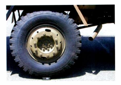
WiNRADiO WR-3700e receiver still functional and without any mechanical damage, after being run over by a "Unimog" army truck (weight approx. 4 tons).
