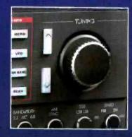
Ultra fine-tuning cf 50Hz on LSB/USB, 100Hz in SW, AM and Aircraft Band and 20 KHz in FM. • For Fixed-step Tuning: Big, responsive Up/Down tuning buttons.
