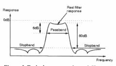
Figure 3 Typical response of a real filter
