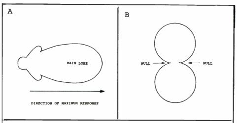
Fig. 1. Radiation and reception patterns for some antennas which can help reduce noise. A beam antenna (A), and a table-to loop antenna (B).
