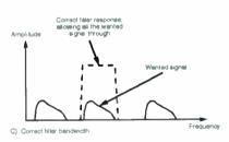
Figure 5 Using the correct filter bandwidth
