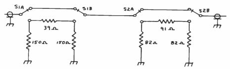
Figure 5. Switched circuits not only allow the attenuator unit to be inserted in the feedline permanently, but you can use fewer networks to achieve the same attenuation.
