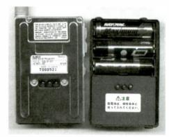
Figure 3. Rear view of DX-X2T (left) and the snap on, auxilliary battery pack/charger (right).
