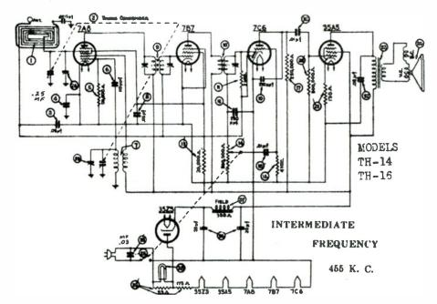
Sorry! The TH14 schematic in my Rider's Manual is a bit blurred. Speaker field (marked "FIELD") is the coil at right of 35Z3 rectifier tube (near bottom of schematic).
