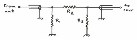
Figure 1. This simple attenuator uses three resistors in a pi-network.
