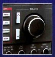
Ultra fine-tuning of 50Hz on LSB/USB 100Hz in SW, AM and Aircraft 3and and 20 KHz in FM.
