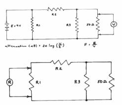
Figure 4(a). Attenuation level can be checked using a battery and a voltmeter. Note that the receiver is replaced with a 50-Ohm resistor. Figure 4(b). Network resistance can be checked by placing an ohmmeter across R1. Note that the receiver is replaced with a 50-hm resistor.
