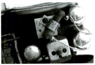
Power resistor clipped to top of speaker frame replaced field coil when original dynamic speaker was swapped for a "PM" unit (see text).
