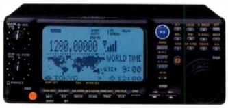
sports a wide variety of scanning capability. The VR-5000 will receive all modes: CW, LSB/USB/AM/AM-N/AM-W/FM-N/FM-W.
