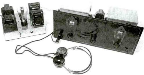
Shot from my original Popular Electronics restoration article shows set as it was set up for testing. Power supply is home built, but based on Pilot K111 circuitry.
