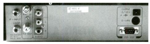
There's not too much to do to get these receivers up and running. An LNB loop-through and video and audio output are all that are needed. There's even room for an outside TV antenna input.
