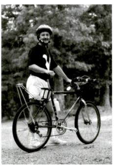
1994 I'm racking up the miles going bicycle mobile, 21 gears no waiting! Note homebrew antenna support structure on back, motorcycle battery power supply under the seat, Alinco 2 meter mobile rig (up to 50 watts out!) and homebrew helmet mounted mike with pushto-talk mounted on the handle bars.
