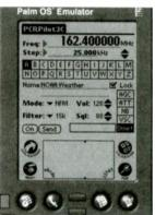
be stored and recalled with a touch of the let-Each ter. memory also can contain a user inputted description of the stored frequency. In Figure Two, we can see that 162.4 MHz is "NOAA Weather." This is the beginning of great things!
