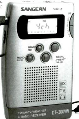
functions, and a memory button. At top center, there is a liquid crystal display that lets you know what's going on with this diminutive receiver and above that, a red light emitting diode tuning indicator. At bottom center, you'll find a roughly once-inch-square grill for the radio's tiny speaker.
