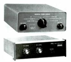
The patch connects to the telephone line. It also connects between a receiver and an external speaker. Phone patches for ham use provide transmitter connections, too, but you can ignore them for scanner applications.
