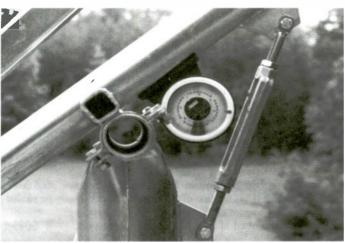
Inclinometer in action, Helps check angles of your dish at the mount, on the pole and on the feed horn. Peaking the dish for optimum performance is easy and can save a service call. (Courtesy Ken Reitz)
