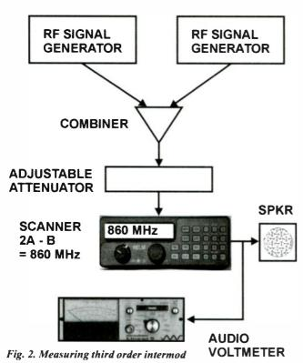
Transmitters on frequencies A and B produce third order intermod signals two frequencies, 2A - B and 2B - A. For example, a NOAA weather transmitter on 162.55 MHz (frequency A) and a paging transmitter on 158.7 MHz (frequency B) may overload your scanner, producing a horrid intermod mixture of weather forecasting and paging tones on 166.4 MHz (2A - B) and 154.85 MHz (2B - A).
