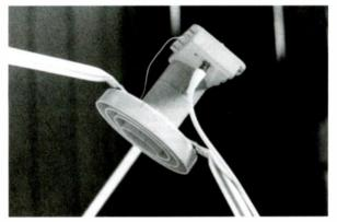
Photo 2. Early LNBFs like this one from California Amplifier used a small wire to deliver the voltage to electronically switch polarity.
