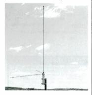
good antenna and match is the secrettogetting maximum range. When we say match we mean electrical impedance match... if the proper impedances are not maintained between transmitter and antenna, power is reflected back away from the antenna and back into the transmitter! This can cause the final amplifier stage to be damaged, not to mention a spurious signal and lousy range."
