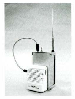
Figure 2. Here's a view of the completed BBB-4 ready for action. I used two strips of Velcro® to attach the outboard speaker-amplifier to the front of the case, and a short patch cord to link the BBB-4 to the amplifier input. (Photo by Chuck Bliley, NY).
