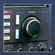
The Tuning Contro s • For the traditiona ist: a smooth, precise tuning knob, produces no audio muting dur ng use. \_ltra fine-tuning of 50-lz on LSB/USB, 100Hz in StV, AM and Aircraf: Band and 20 KHz in FM.
