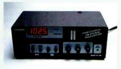
Unlike many lower power transmitters that depend on "wall wart" or battery power supplies, the FM-100 has its own internal power supply. This supply benefits from filtering capacitors to reduce ripple, eliminating background audio hum. All your listeners should hear are your broadcasts.
