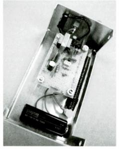
Figure 1.. It's not fancy, but it does the job. This view shows the circuit board and other parts mounted inside an aluminum enclosure (Photo by Chuck Bliley, NY).
