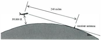
Fig. 2: Typical horizon at 39,000 feet.
