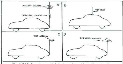
Fig. 1. Vehicular antennas with inductive and capacitive loading (A), with ideal mounting in the center of the vehicle's roof (B), of the halo design (C), and of the big wheel design (D).
