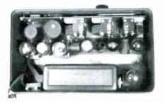
FIG. 2. Interior of the AK 42. Power supply is oblong box at bottom of picture.
