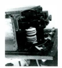
Close-up of spark gap which forms the spark. The large size of the gap is to facilitate cooling.
