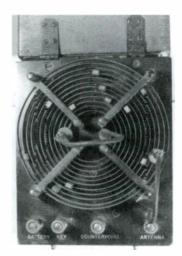
BC-15A, Airplane Radio Telegraph Transmitting Set Box, looking at top of unit.
