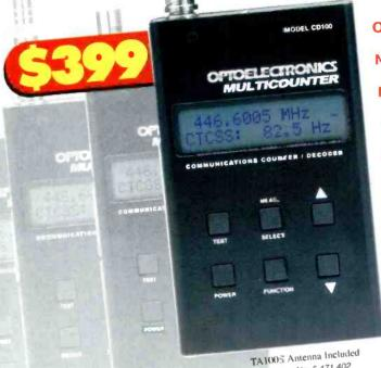
Multicounter CD100 Counter / Decoder. The Multicounter combines a frequency counter and tone decoder in one handheld package. As the Multicounter locks onto a nearby RF signal, the frequency along with either CTCSS, DCS, LTR, or DTMF is instantly shown on the two-line LCD display. Like the popular Optoelectronics Scout, the
