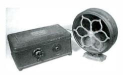
FIG. 1. Atwater Kent Model 42 is a good example of an early (1927) plug-in set. It used a separate speaker just as did the early battery sets. Note uncluttered front panel.
