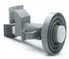
ADL RP3-CKU international C/Ku-band feed horn has capabilities to receive linear and circularly polarized C-band signals and is characterized by extra length in the C-band wave guide and built-in Teflon inserts. Provides better performance over simple insert. (Courtesy ADL)
