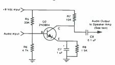
Fig. 2. Audio Preamplifier
