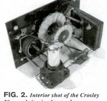
FIG. 2. Interior shot of the Crosley 50 reveals its simple, sturdy construction.
