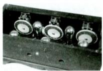
FIG. 4. A peek inside the set of Fig. 3 shows the set of five 01-A tubes and the three tuned circuits.
