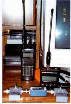
The Icom 32A shown with its computer interface cable plugged into the speaker jack. Alongside are my trusty Optoelectronics Scout and its FM and VHF paging filters.
