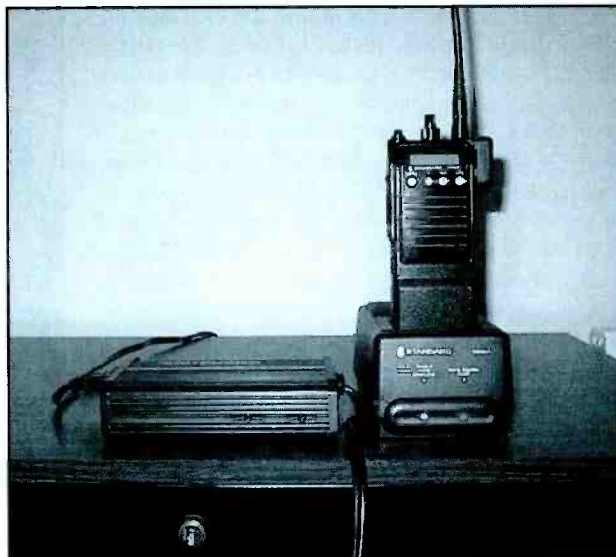
Standard two-way radio charger plugged into a Statpower 250 watt inverter
