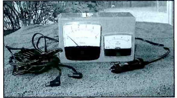
A combination volt and ammeter power 12 volt power distribution box.
