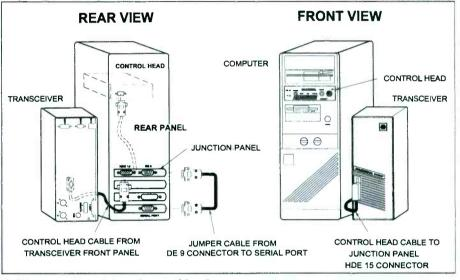
Cable connections, internal control head
