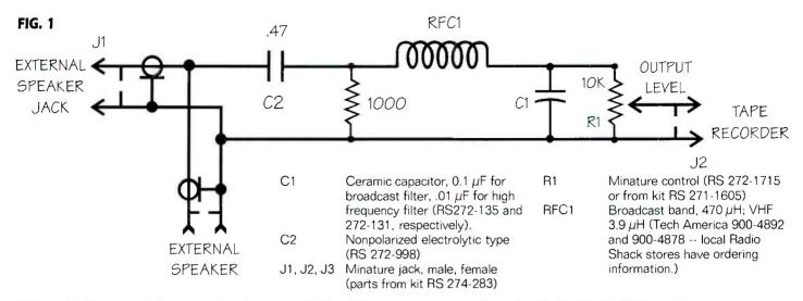
Schematic diagram of the audio interface and rf filter. RS part numbers are from the Radio Shack 1998 catalog.
