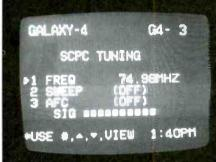
A video tuning feature allows the user to make adjustments to improve picture quality which is useful when experiencing Terrestrict Interference (TI) on C-band or narrow band video on Ku-band.
