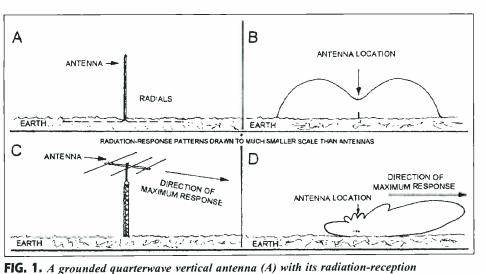
patterning (B), and a Yagi-Uda beam mounted a half wavelength above ground – with its
