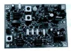
FIG 3. The actual circuit board for the SW-40+ transceiver. Don't let the small size and low parts count fool you!
