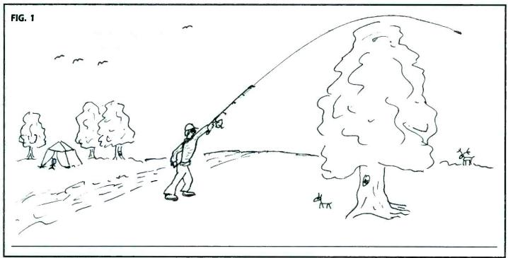
One method of getting a line over a tall tree for vacation-antenna erecting.
