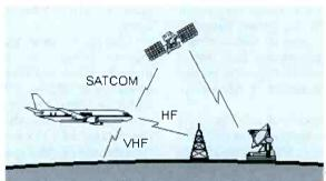
moting GLOBALink, which attempts to extend the line-of-sight range of VHF ACARS. The goal is to seamlessly integrate VHF with HF and satellites, switching modes as necessary. This has required adapting ACARS to the more demanding conditions of noisy HF links.
