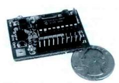
FIG 4. NN1G's FreqMite digital frequency readout board will make most rigs into a digital readout radio. The frequency is sampled and read out via Morse code at either 13 or 26 wpm. This little board fits nicely into the SW-40+ custom case.
