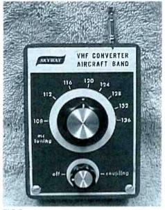
FIG 2. Old Skyway converter allowed VHF air band reception when placed next to a broadcast receiver (photo by R. Lucchesi, WA2ROY)
