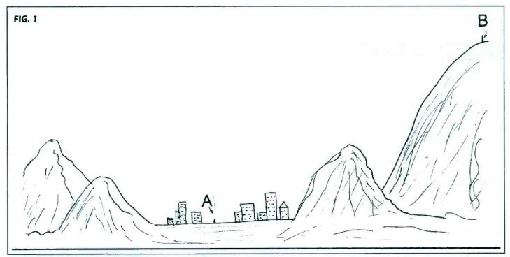
Communication paths from the rubber-duck antenna on the HT located at A are very limited by buildings and terrain, but the paths possible for that same signal repeated from the antenna at B allow much greater coverage.
