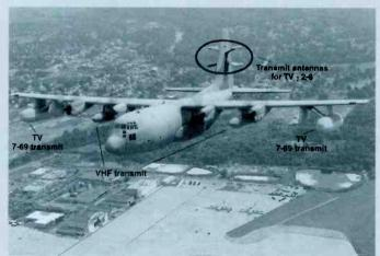
An EC-130 flying over its base at Harrisburg. Duplicate sets of TV antennas allow the operators to choose the set facing the target.
