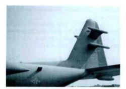
Close up of HF receive antenna (above) and UHF/VHF antenna (below).
