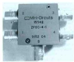
FIG 1. Mini-Circuits ZFSC-4-1 four way splitter worked well from 500 kHz-1000 MHz.
