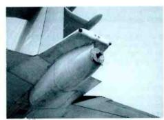
The HF antenna pod from which the wire antenna is deloyed.
