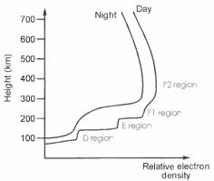
FIG. 2 The approximate levels of ionization in the ionosphere
