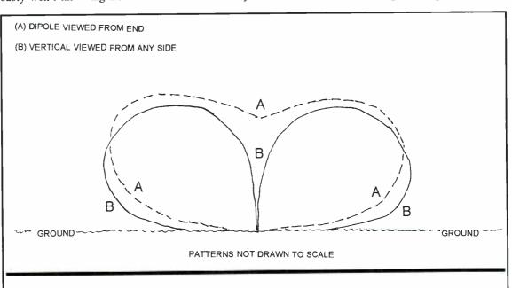
choice. NVIS is produced by an antenna which di- (A), and a ground-mounted, quarterwave vertical antenna (B).
