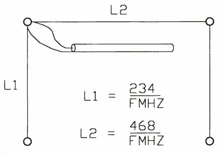
5 in. of wire to each vertical section to bring resonance to 7.1 MHz. This may be due to the proximity of the feed end to just a few inches from my metal tower.
