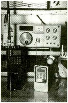
The Alinco DJ-C1 is on the right and my trusty Icom IC-24AT is on the left (for size comparison). The DJ-C1 has the optional speaker mic attached. This little HT does double duty as a 2 meter rig and a VHF scanner with air band.
