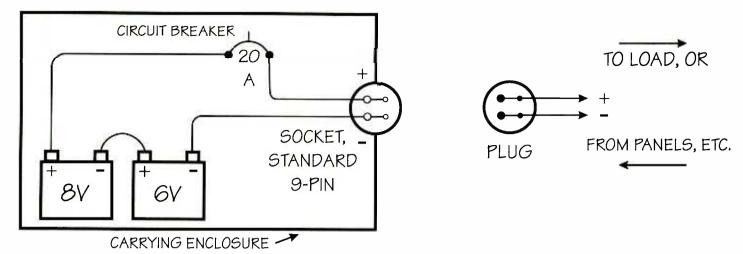
FIG 1. Typical 14V power pack, one of two or more identical units
