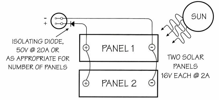
FIG 3. Two solar panels 16V each at 2 amps with isolating diode.
