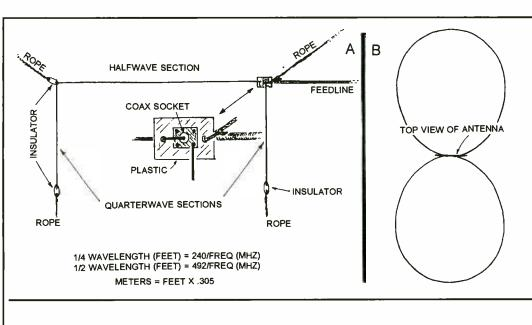
FIG. 1. A half-square beam antenna (A). The antenna's horizontal radiation-reception pattern (B).
