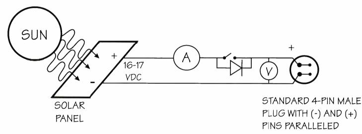
FIG 2. Simplified charger box showing metering and optional diode bypass switch
