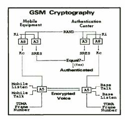
ing. The SIM card sends RAND and the secret 128-bit key Ki through the A3 algorithm to produce a 32-bit "signed response" (SRES). This number is transferred out of the SIM into the phone, where it is then transmitted to the network. This is the phone's response to the network's challenge.
